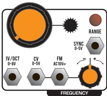
This block is the internal oscillator control. The large knob and small shaft are the coarse and fine tune controls. The "range" button switches between audio and LFO mode, the latter being the RED color. The attenuverter is shared between the "CV" and "FM" inputs. CV is a unipolar, exponential frequency input, and FM is an AC-coupled audio input for thru-zero frequency modulation.
